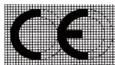
Fig 2: CE mark for a device where a notified body is not involved in the assessment of the device
