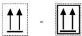
Two black or red arrows on white or suitable contrasting background. The rectangular border is optional
