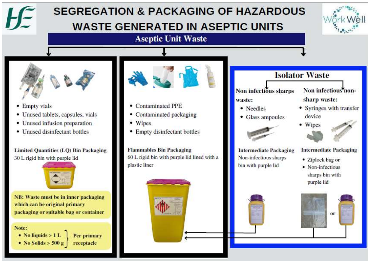
Figure 2 Segregation and Packaging of Hazardous Waste Generated in Aseptic Units
